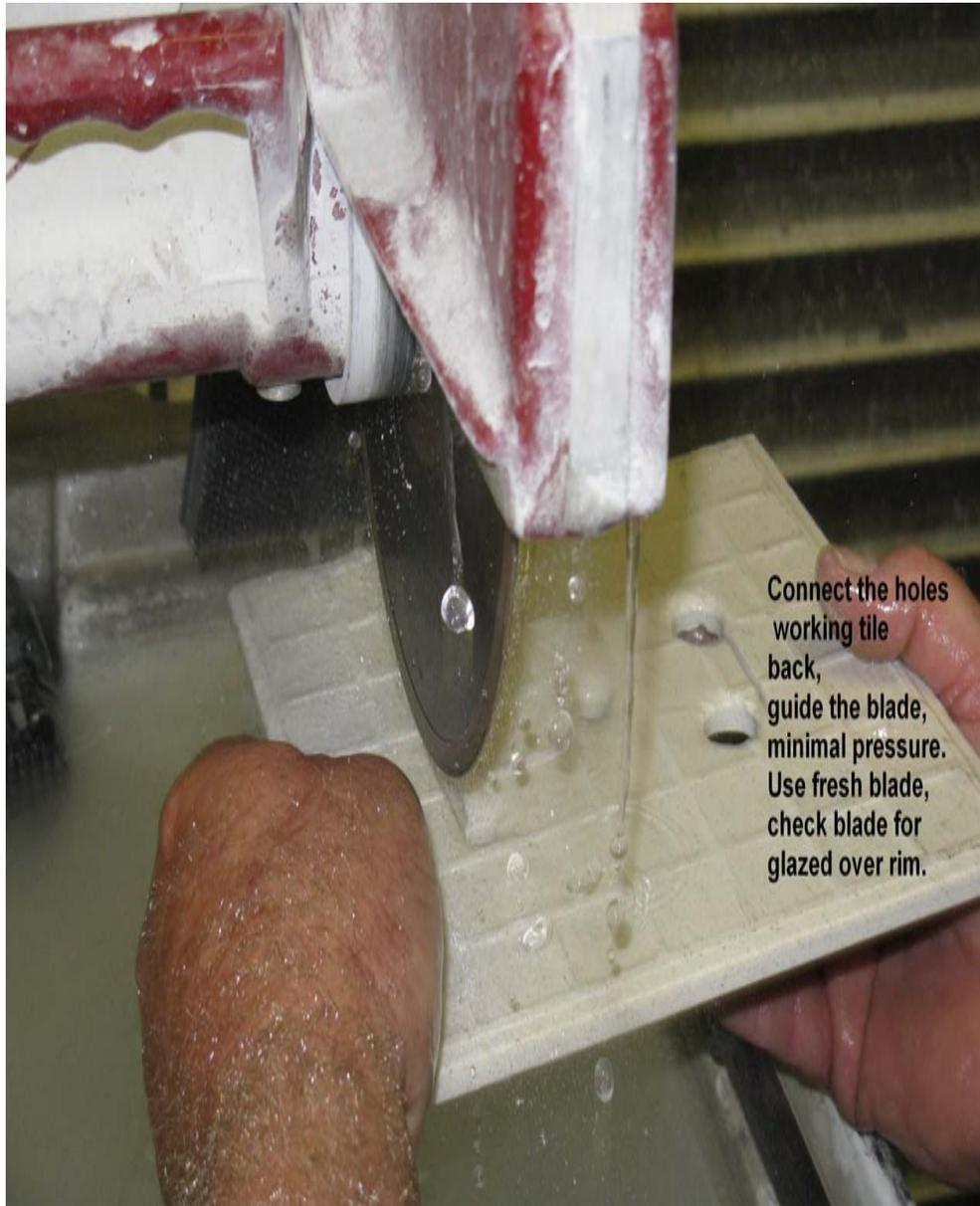
Connect the holes working tile back, guide the blade, minimal pressure. Use fresh blade, check blade for glazed over rim.
